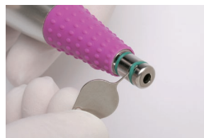
Replacing O-rings on the Outer Sheath
