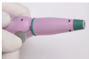
Replacing O-ring on the Motor Component
