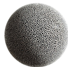
Fig. 1 Schematic illustration of a spherical mesoporous nano-silica used in BioArmor. Average particle size: 450 nm, the pore size is 1–2 nm.
