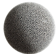
Fig. 1 Schematic illustration of a spherical mesoporous nano-silica used in BioArmor. Average particle size: 450 nm, the pore size is 1–2 nm.
